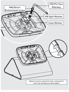
Attach the Shell to the Flip. Take care to ensure correct & full thread engagement.
