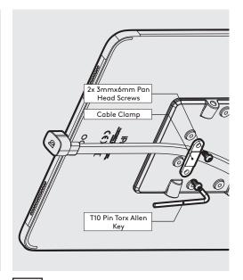
Secure the Flat Cable to the Mounting Plate with the Cable Clamp as shown.
