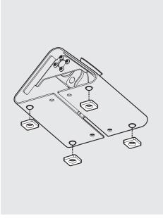
If wishing to slide your Flip across your mounting surface, apply the supplied Felt Feet as shown.
