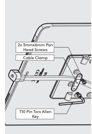
Secure the Flat Cable to the Mounting Plate 6 with the Cable Clamp as
