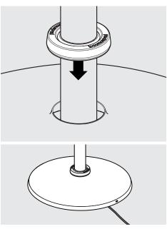
With the Floorstanding Cover on the ground, locate & fit the Floorstanding Rubber Collar.
