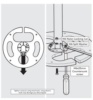
Orientate, locate & secure the Floorstanding Pole to the Floorstanding Base as shown. Ensure that all fixings are installed correctly.
