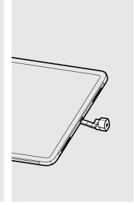
Attach the Flat Cable 5 to the Tablet with the U-Bend Head.
