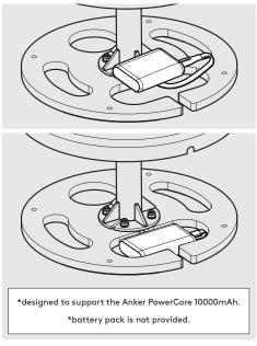
9.2 If installing a battery pack, connect the Tablet Cable and locate the pack into the Floorstanding Base.
