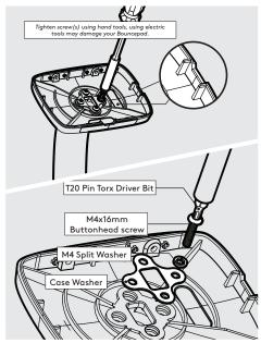
Locate & attach the Shell to the Floorstanding in the correct orientation.
