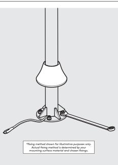
Secure the Floorstanding Pole to the mounting surface, using your chosen fixing method.
