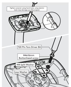
Locate & attach the Shell to the 5 Floorstanding in the correct orientation.
