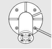
Mark the drill hole 2 locations on the mounting surface.
