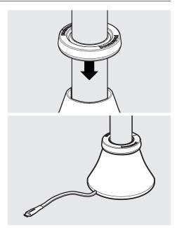
With the Floorstanding Slim Cover on the ground, locate & fit the Floorstanding Rubber Collar.
