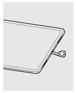
Attach the Flat Cable to the Tablet with the U-Bend Head.
