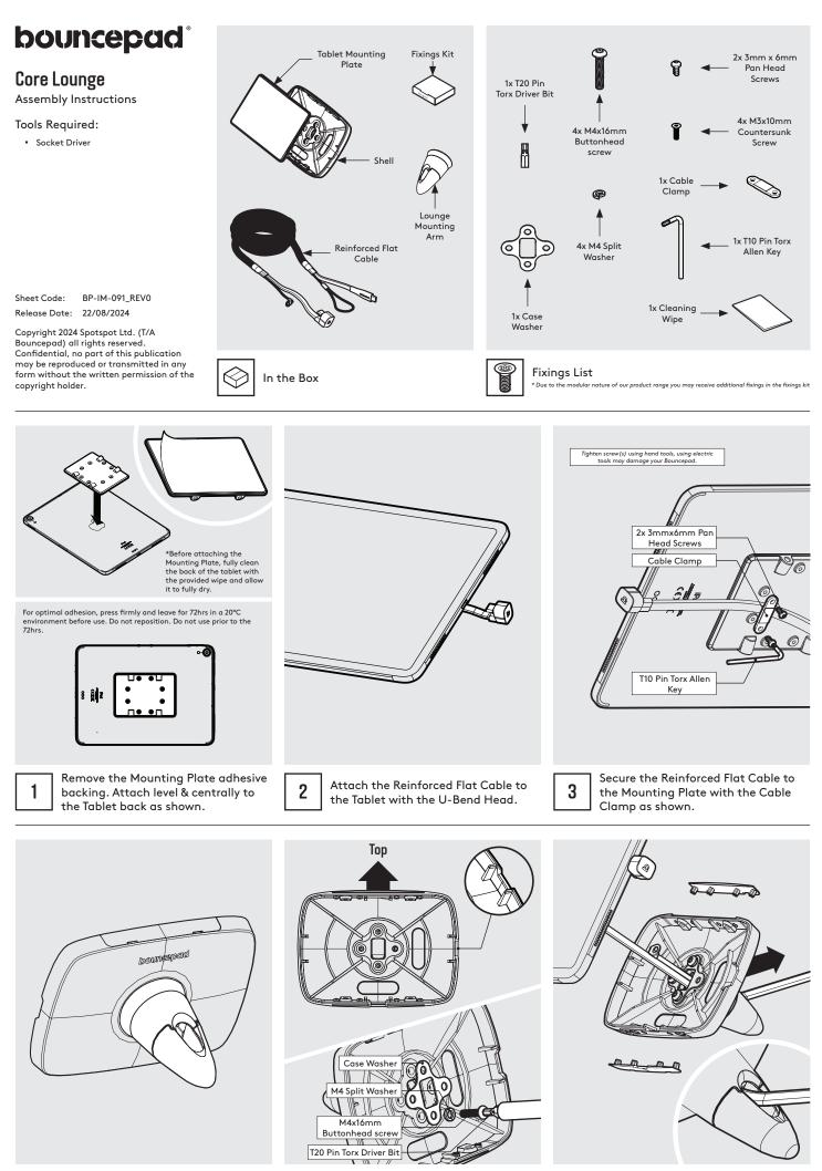
Ensure the Lounge Cone is orientated correctly as shown, with the cable exit at the top.
