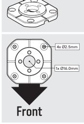
Using the Mount Plate, mark the drill hole locations as shown.
