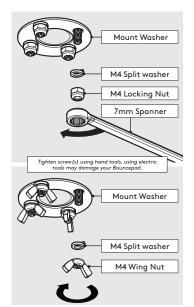
Secure the arm to the A4 surface. Locking Nuts offer higher security.
