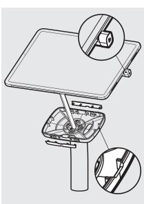
Remove the Fixing Covers. Feed the Flat Cable into the assembly & locate the Tablet in the chosen orientation.
