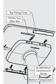
Secure the Tablet to the 6 Shell & attach the Fixing Covers as shown.
